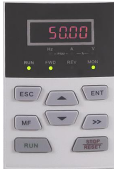
Fig. 4-3 Run parameter display status (Displaying run frequency – 50.00Hz)
